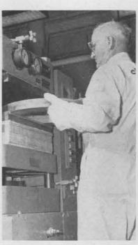
FIFTY-TON COMPRESSION molding press is operated by Harold W. MacGregor. Plastic and rubber are molded under heat and extreme compression.
